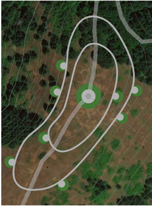
Fig. 5.23: Summit is leveled around the sculpture with two entrenched paths circling it. Observation nodes orbit the paths and remain at a 2 percent grade.
